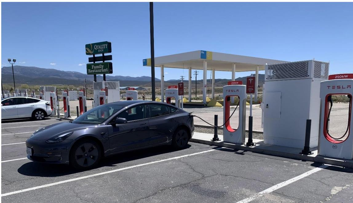
Level 3 Tesla Supercharger station in Beaver, Utah, with up to 250kW charging.
