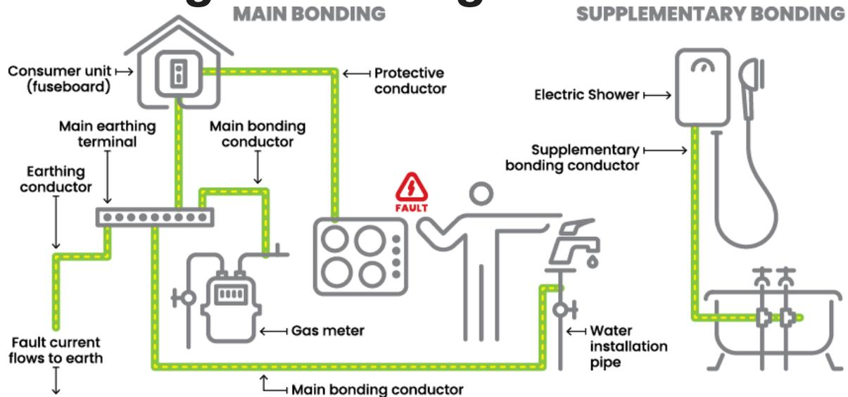
Earthing and bonding must be implemented in accordance with BS7671 to ensure the safety of the wiring installation. Both earthing and bonding uses the yellow and green wire colour coding.
