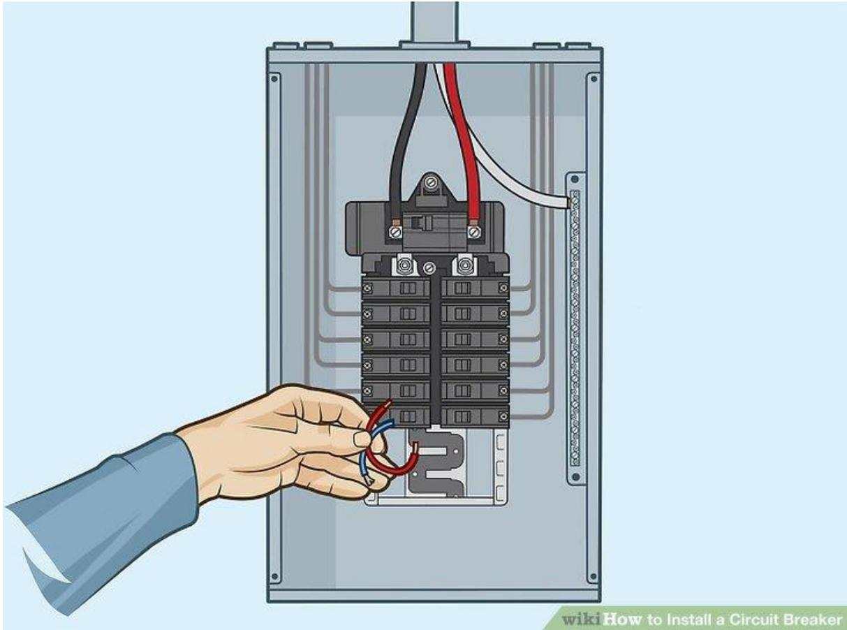
**Clean all foreign objects out of the panel and reinstall the cover.** Remove any tools, wire scraps, or other foreign objects that could cause a short circuit from the interior of the panel. Then, place the cover on the panel to check that the circuit breaker has fully been seated at both contact points and fits through the cover. Finally, rescrew the cover onto the panel.[\[10\]](#)
