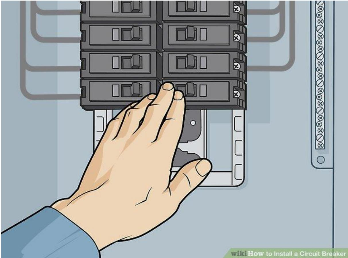
**Firmly press on the circuit breaker to seat it onto the bus bar.** Use your thumb to press firmly but gently on the circuit breaker until it snaps into place on the bus bar. You don't have to screw the breaker into place; it's held in place by spring clips and the panel cover.[\[7\]](#)
