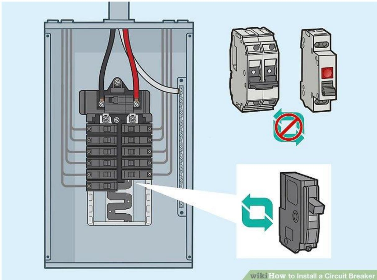
**Make sure you have the correct circuit breaker.** The panel label will list all the approved types of circuit breakers that can be installed in the panel. Deviating from the list is a code violation and voids any UL, FM or other listing services' approval. For maximum safety, use only those circuit breakers that are allowed to be installed in the panel.<sup>[5]</sup>
