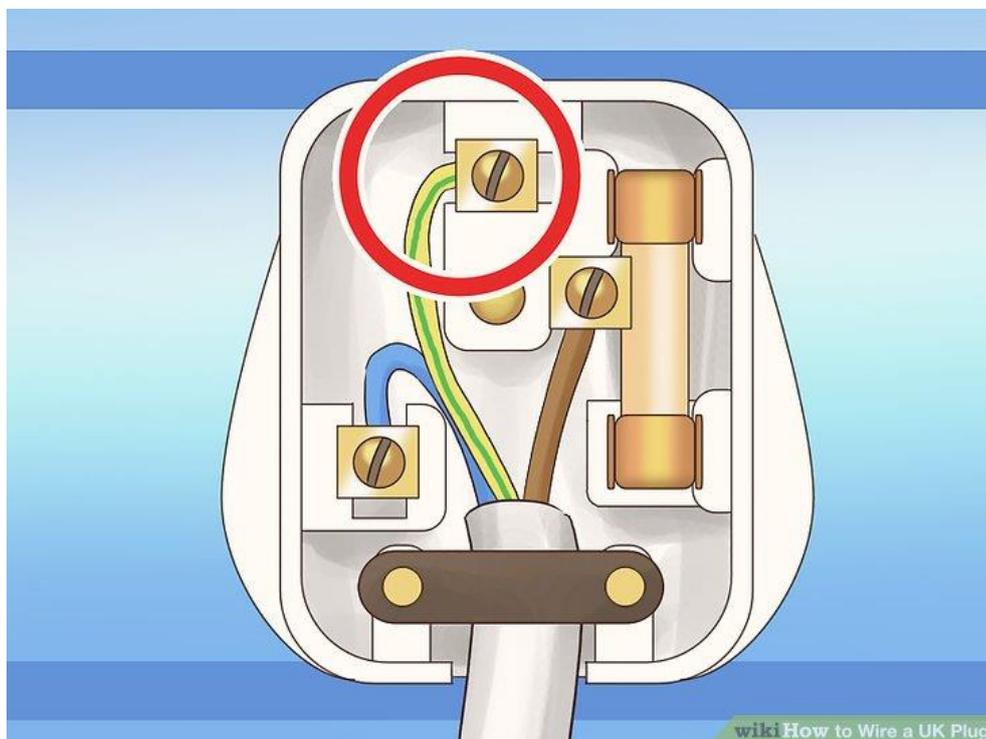
The green and yellow wire is the earth wire, and goes through the middle up to the hole in the top.
