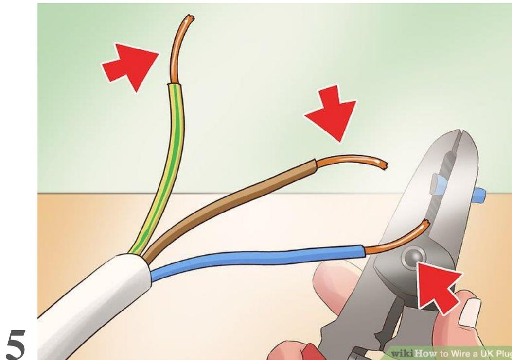
Strip roughly 0.5 to 1 centimeter (0.2 to 0.4 in) off of the end of the blue, brown and striped wires, so that the copper insides are clearly visible.
