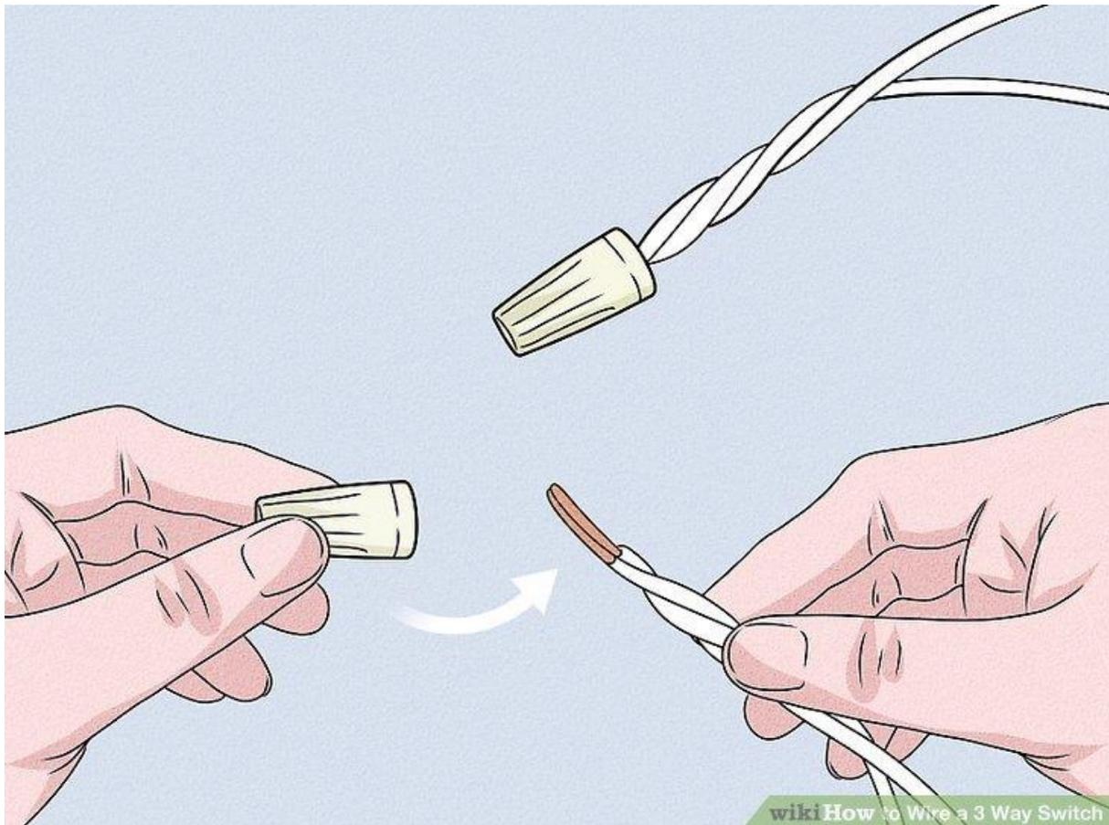
**Cap the equipment grounding conductors together at each switch and the light.** Find the grounding screw on the top or bottom of each of the switches. Wrap the wires tightly around the screw and use a screwdriver to tighten the screws. Cap the grounding conductors at each switch box. Push the wires into the back of your box.
