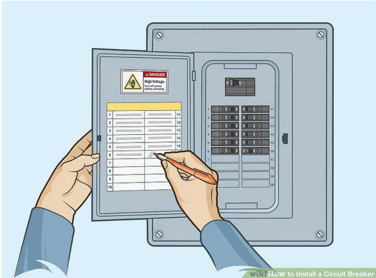
**Label the circuit breaker.** Locate the panel's *circuit directory* on the inside of the panel door. Determine the circuit breaker location (or "circuit number") and write a description of the circuit (load type such as "refrigerator" or a location such as "living room") in the space provided. Be sure to edit the directory if any circuits were moved to install the new circuit.<sup>[12]</sup>
