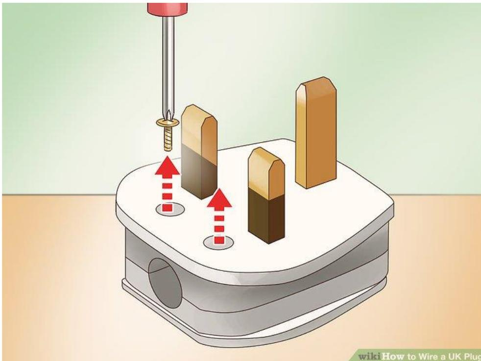
Undo the Philips screw in the center of the plug, on the side with the three pins poking out.
