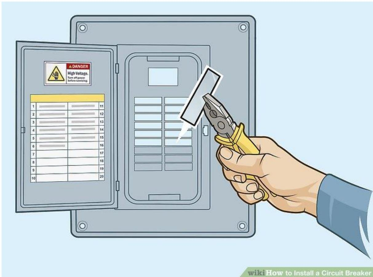
**Remove knockout plates from your cover as needed.** Bring the cover up to the panel to compare the new circuit breaker location to the cover openings. Use a pair of pliers to remove any knockout plates on the cover location where the circuit breaker will be located.
