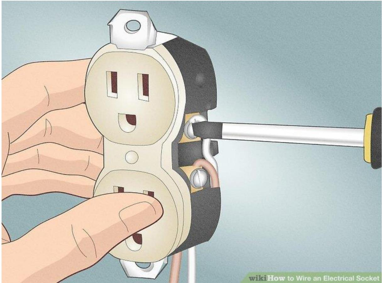
**Tighten the terminal screws.** Use a screwdriver to tighten each screw until it presses down against the wire. Tighten enough for a firm connection, so the wire cannot get jostled out of place, but don't tighten with maximum force.
