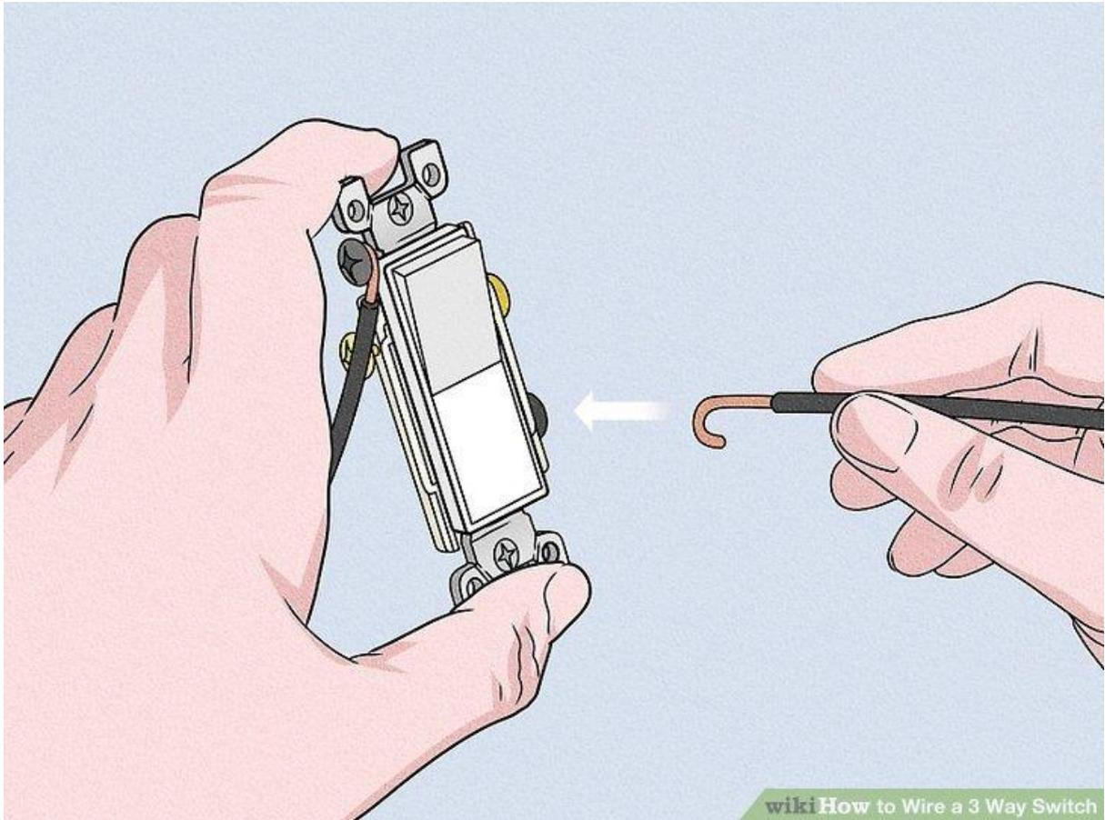
**Connect another black wire from the light to the original switch location.** Use the existing 2-wire conductor leading from the light to the switch. Attach the wire to the black common screw on the switch.
