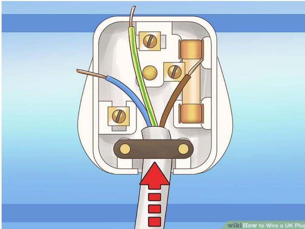
Put all three wires through the cable grip, along with the thick white cable, until the cable grip can be securely tightened onto the thick white cable. The cable grip may have to be loosened with a Philips screwdriver in order to fit the cable underneath it.<sup>[2]</sup>
