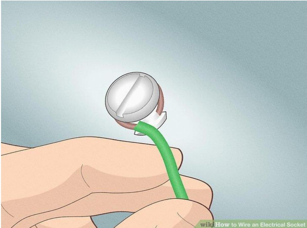
**Wrap the wires around the screws clockwise.** Each wire should rest snugly around its terminal, with all three sides of the U-bend in close contact. Wrap them in the direction the screw tightens (usually clockwise) for maximum contact with the screw threads.<sup>[18]</sup> Before you do this, be about 700% sure you are using the correct wire:
