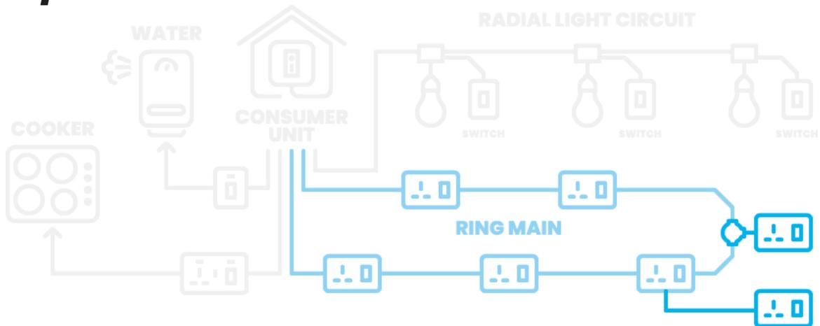
Spur is a short branch of cable from existing ring main circuit. The branch can stem from an existing electrical device or from a junction box as pictured above. Every unfused spur can only supply one socket or connection unit. The total number of spurs cannot exceed the number of devices on a ring main circuit.
