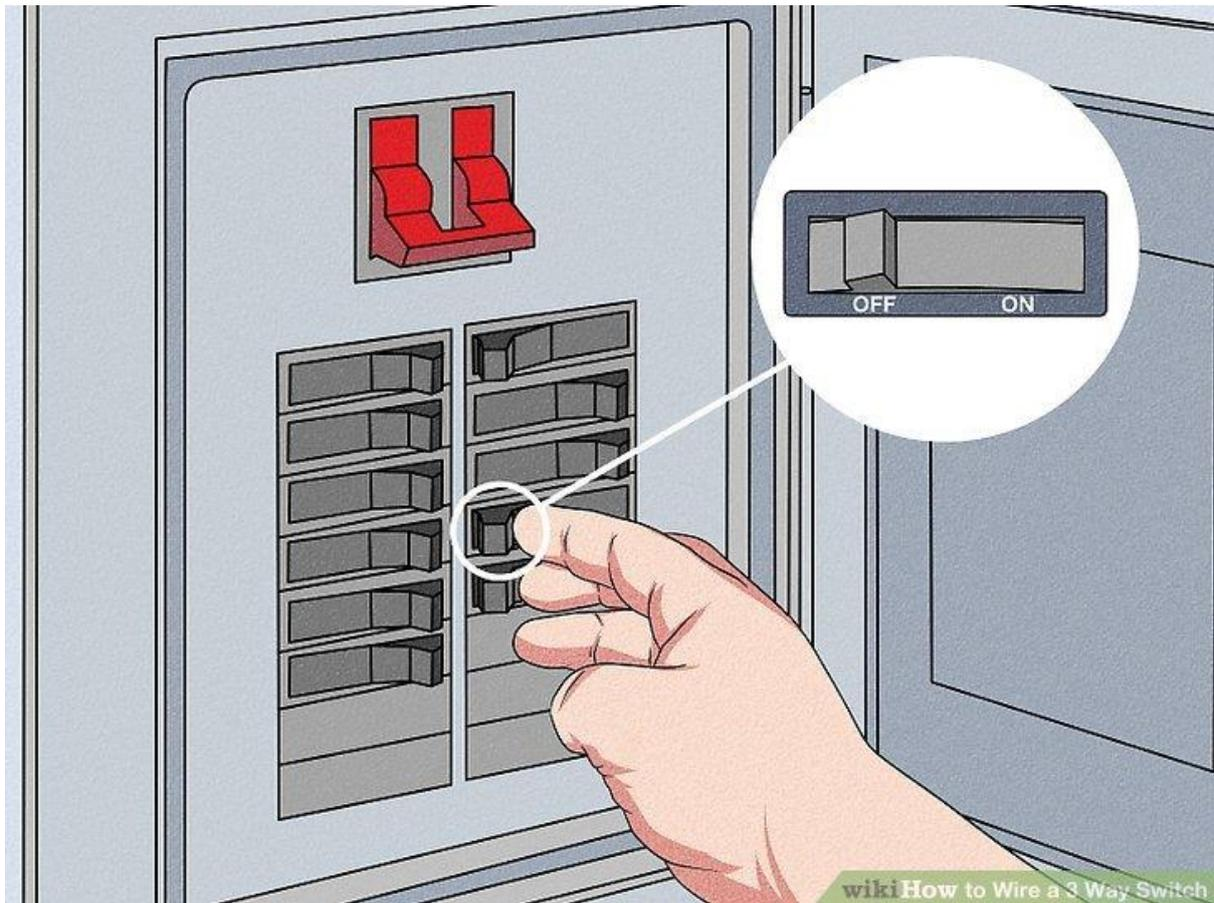
**Switch off the circuit.** Ensure that the circuit for the room you are working in has been flipped off. This will prevent accidental electrocution and reduce the risk of fire.<sup>[1]</sup>
