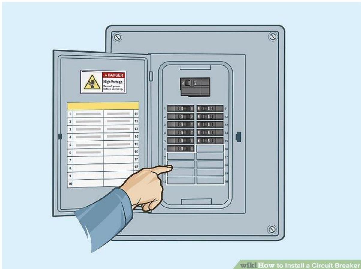
**Inspect the circuit breaker arrangement for unused locations.** Look for a blank area on the electrical panel that could accommodate a circuit breaker, paying particular attention to unused spaces at the top and bottom of the cover. Some manufacturers of electrical panels have removable
