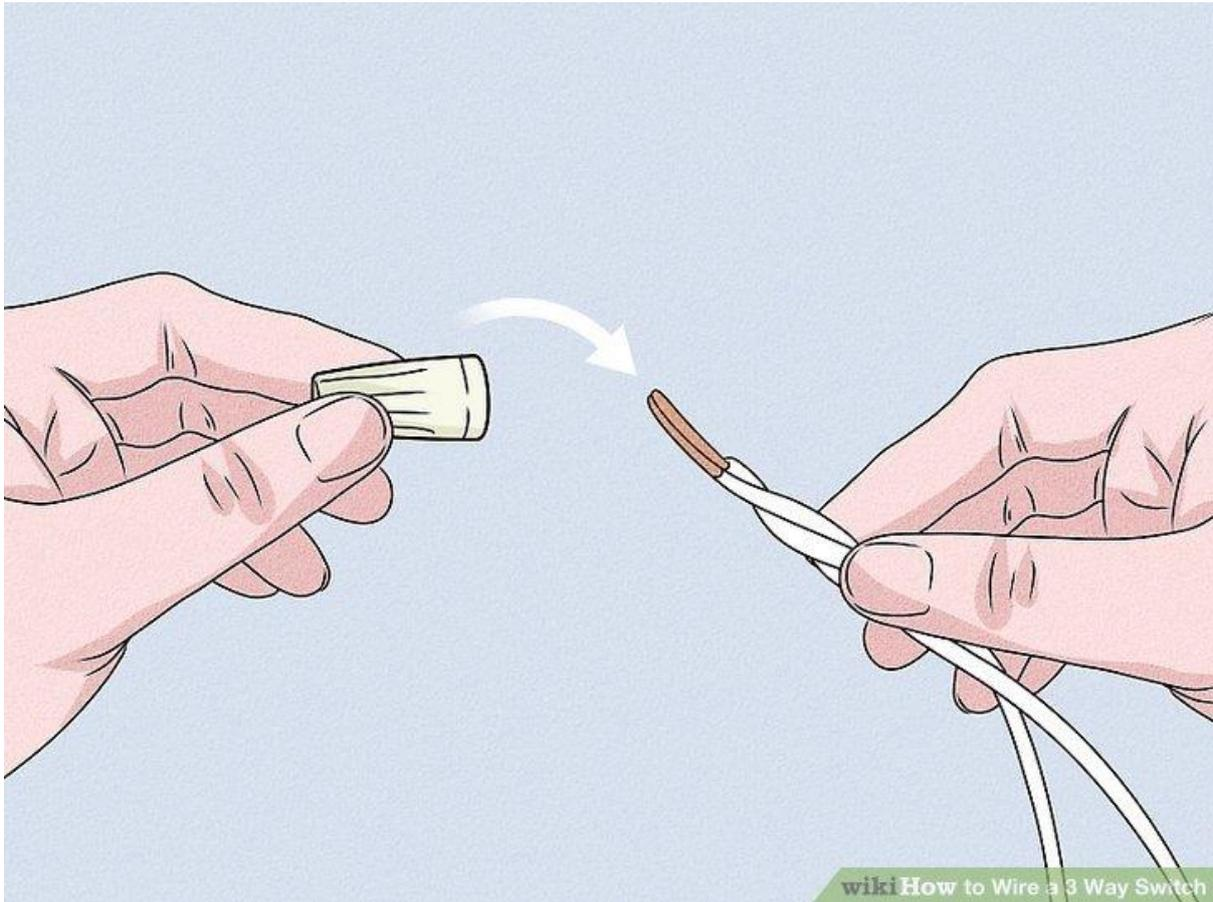
**Cap the white neutral wires to each switch box.** Place a plastic cap on the end of the white wire from the top conductor in the new switch location. Take the neutrals from the other end of the top conductor, the power source, and the light and cap them in the original switch location.
