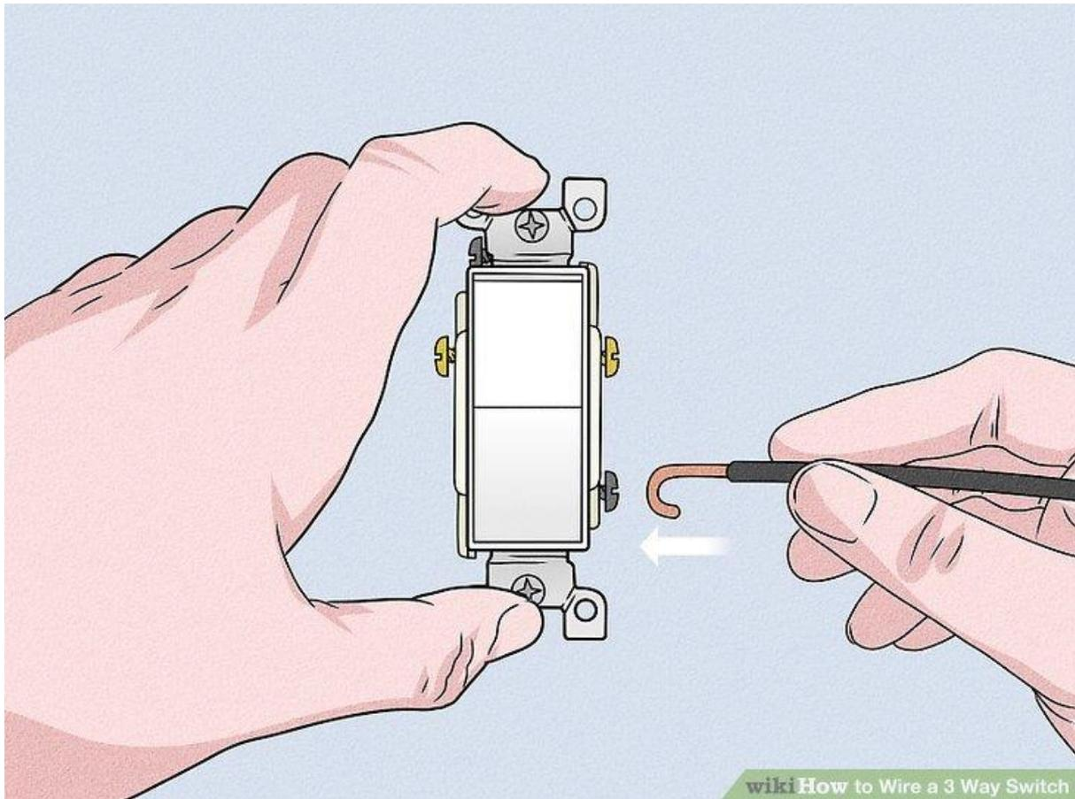
**Run a black wire from the new switch to the power source.** Use the black wire in the top 2-wire conductor to attach the switch to the source. Make a J-hook in the wire with a pair of pliers and wrap it around the black common screw on the light switch. Tighten the screw to secure it in place. Cap the wires connecting the source and the switch.
