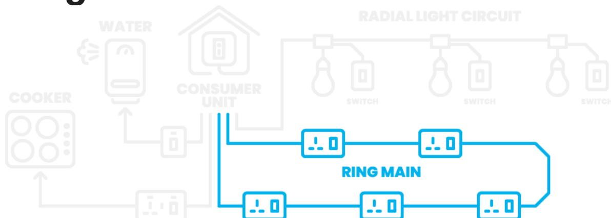
Ring main circuit starts from the consumer unit, connects to a number of electrical devices (typically sockets) and then returns to the consumer unit. Electrical current can flow from either end of the ring.
