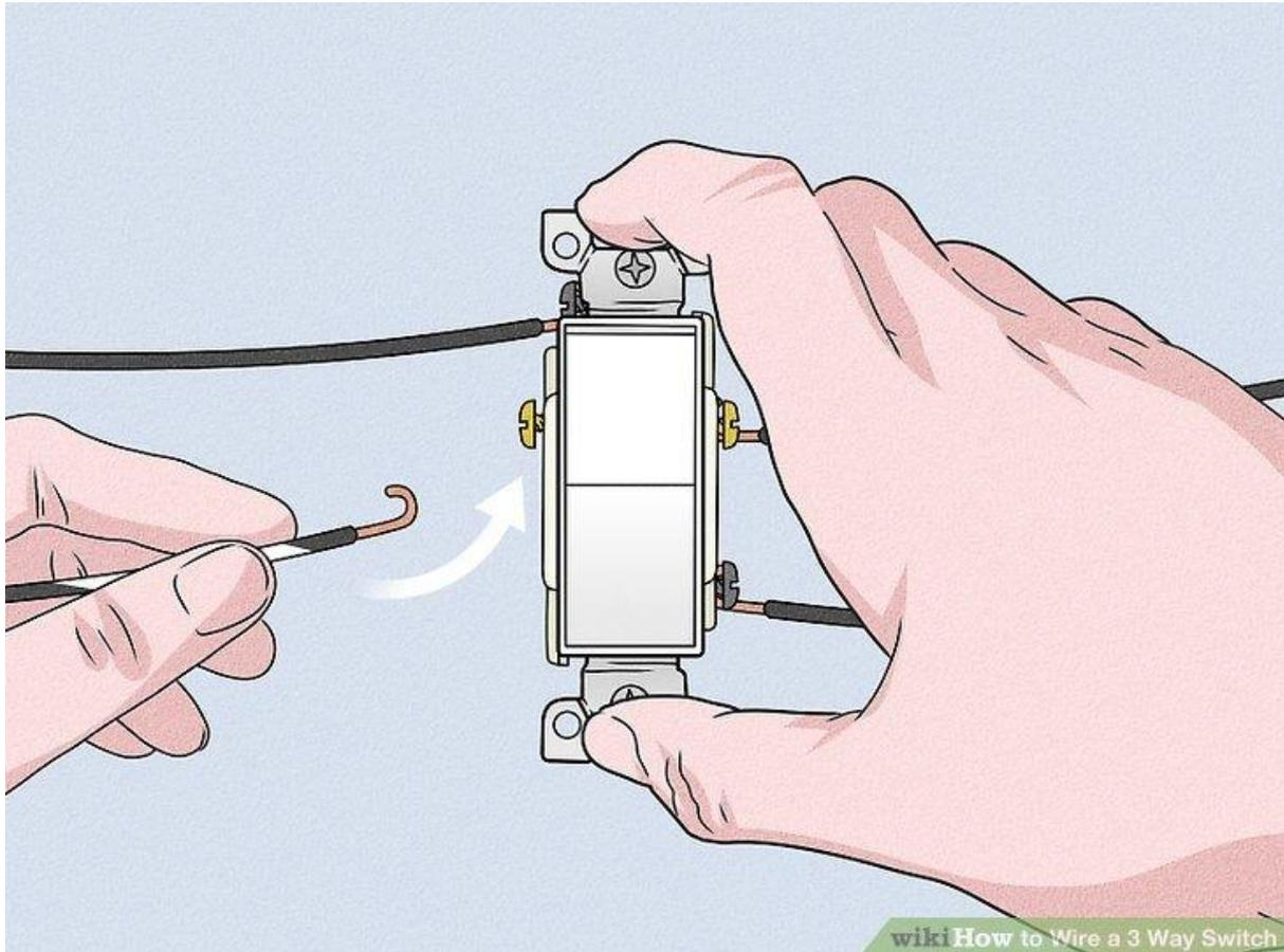
**Connect the traveler wires using the bottom conductor.** Use the black and white cables from the bottom conductor to attach the traveler terminals on each switch. It doesn't matter which terminals they are attached to on each switch. Use a pair of pliers to bend the exposed ends of the wire around each screw.
