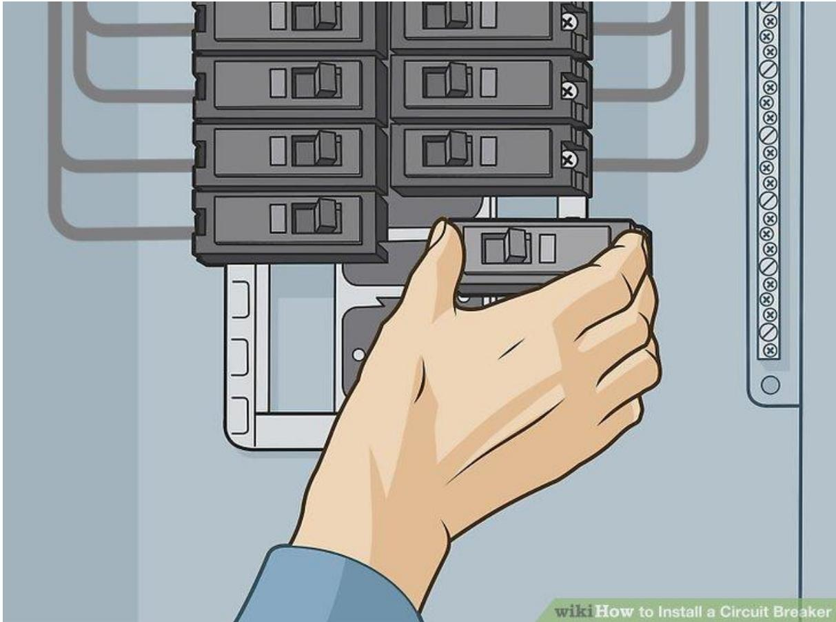
**Align the circuit breaker with the bars in the panel.** Tilt the circuit breaker so that the hold-on clip on the bottom of the breaker is attached to the plastic “grab” bar in the panel. Once attached, pivot the circuit breaker on the mechanical contact and roll towards the center of the panel - making sure the bus bar of the panel is still aligned with the slot or opening on the circuit breaker case.
