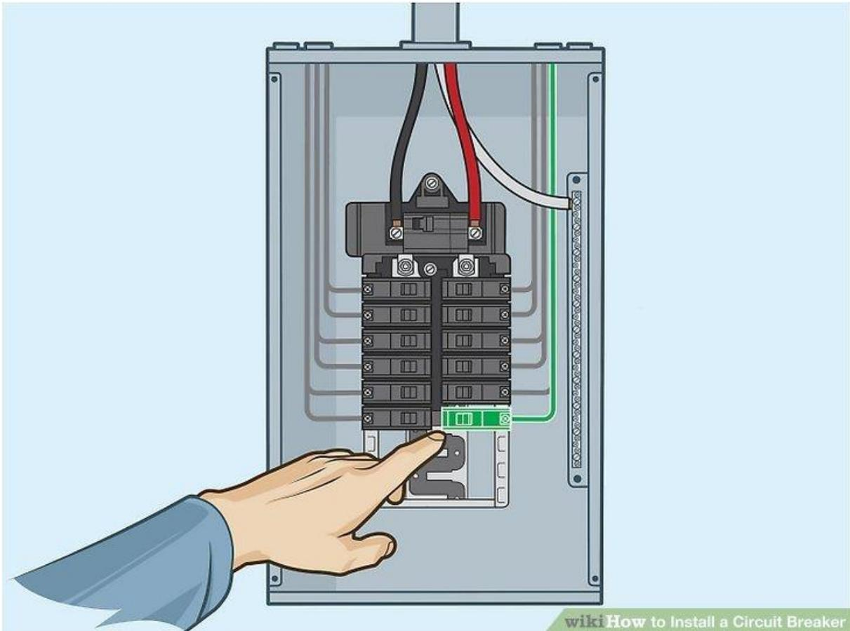
**Find an unused space next to or between existing circuit breakers.** The new circuit breaker you install will need to be placed next to a circuit breaker already in place. Carefully compare this location to the cover that was removed earlier to make sure it aligns with an unused location on the cover.<sup>[4]</sup>
