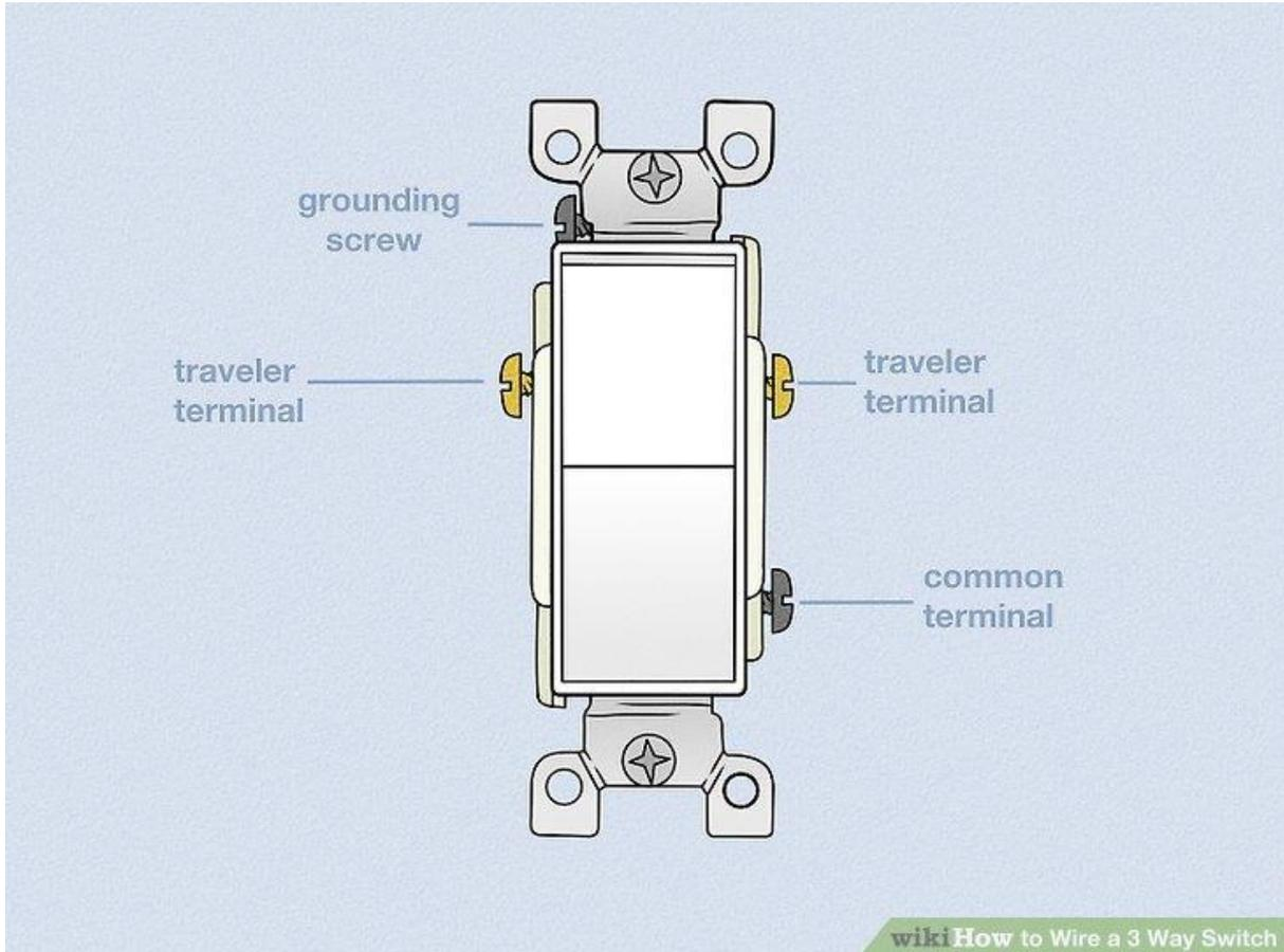
**Replace any regular switches with the 3-way switches.** A 3-way switch will not have the words on or off written on it. Before you start installing, take a look at your new 3-way switch to identify all of the terminals that you will be connecting wires to.[\[2\]](#)
