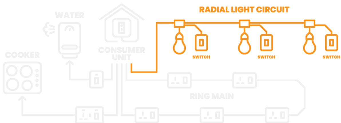
Radial circuit is a single cable run from a consumer unit circuit breaker to a number of electrical devices and terminates at the last device.
