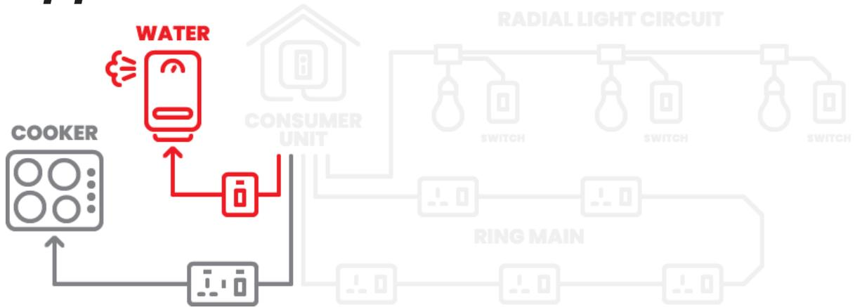
High current hard wired appliance such as cooker, hot water unit and electric shower require dedicated circuits from the consumer unit. These circuits have higher gauge wiring and protected by high rating circuit breakers.
