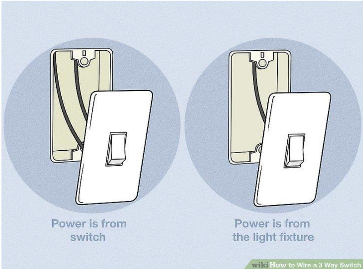
**Determine if the power goes to the light or the light switch.** This will affect the way that you perform the installation. You can tell if the power is coming into the switch by removing the light switch panel. If two black wires are coming into the switch box, then the power is coming into the switch first. If there is only one black wire, then the power is coming into the switch from the light fixture. You can usually use an electrical tester to be sure.
