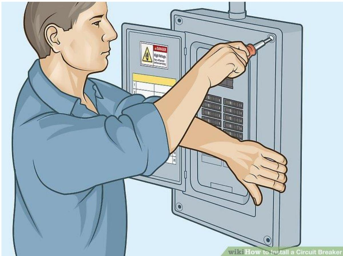
**Remove the electrical panel cover.** Use a screwdriver to remove 3 of the screws supporting the cover. Then, use 1 arm to hold the panel cover in place as you unscrew the last screw. Finally, pull the cover away from the panel.[\[2\]](#)
