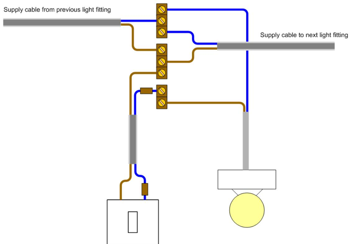
All [cable colours](#) are as expected **except** for the switched live. Light switches are usually wired with standard T&E, which means the switched live wire will be black (existing installs) or blue (new installs) - this **should** be marked with live coloured [tape](#) or sleeving (though alas this is often missing).
