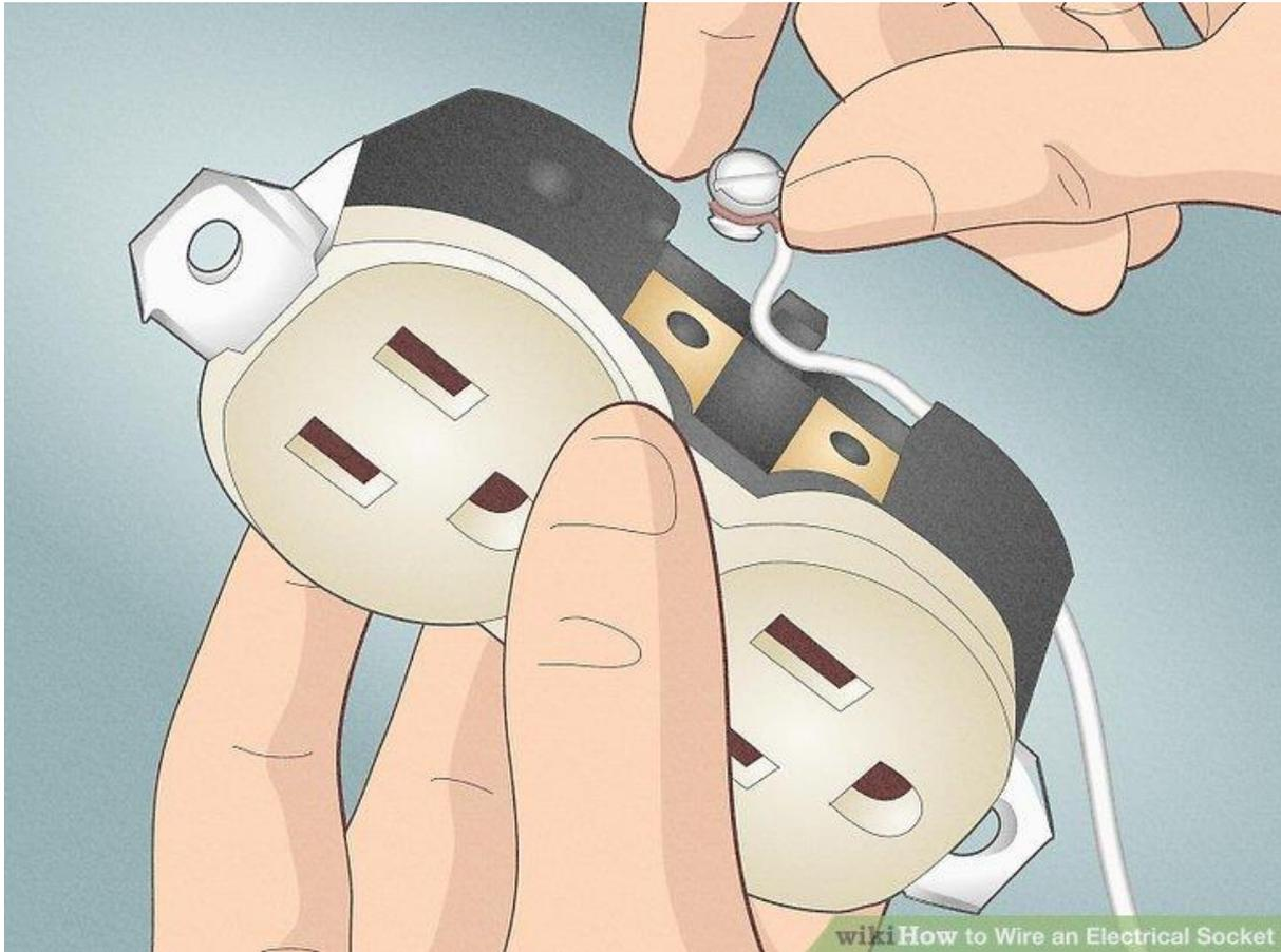
**Tuck the wire under the plastic retainer.** Most outlets have small plastic ledges for you to tuck the wires under to secure them in place. If this isn't working well, double-check the wire stripping:[\[21\]](#)
