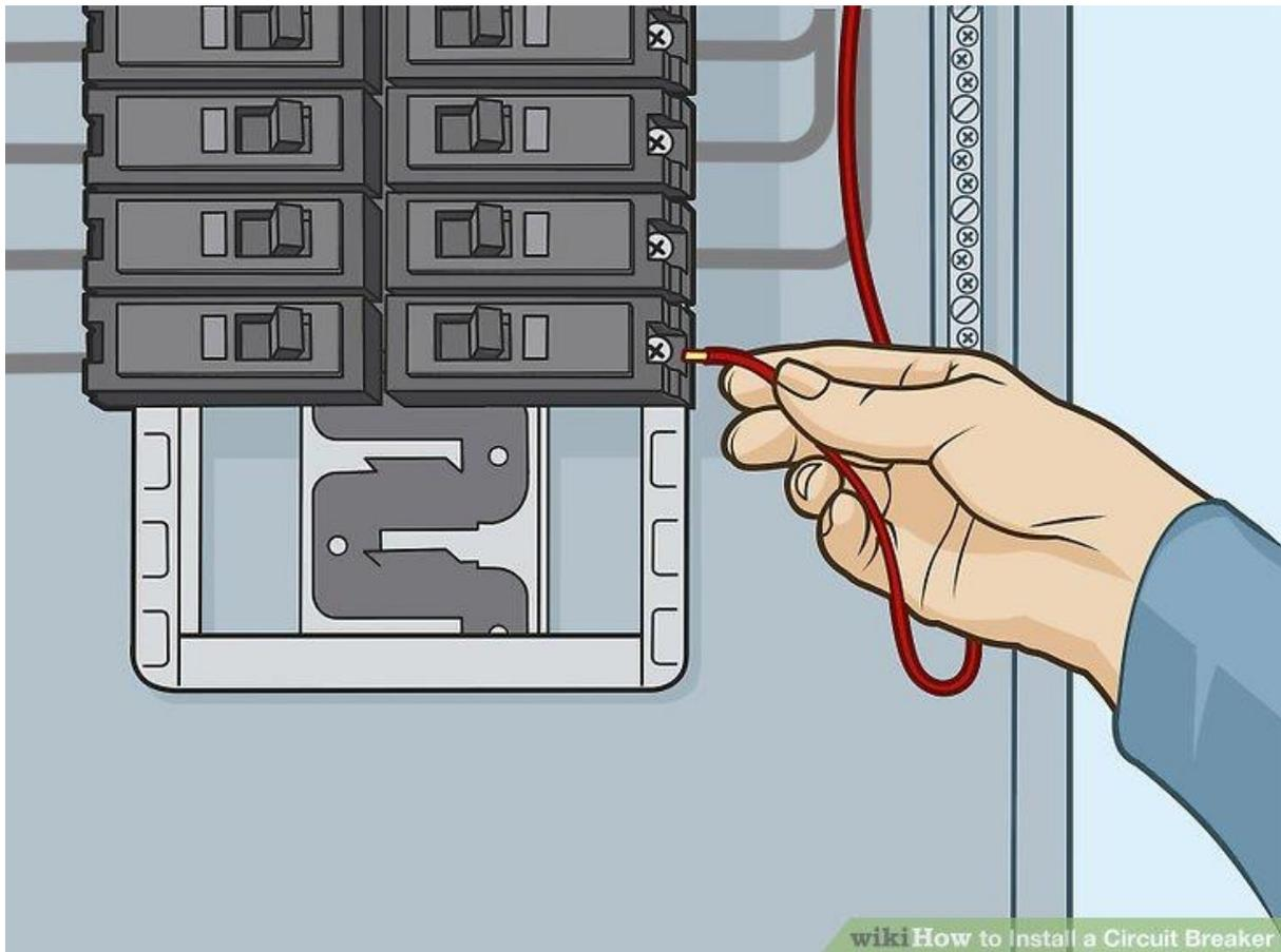
**Connect the circuit wiring to the electrical panel.** After making sure the circuit breaker is still in the OFF position, connect the white neutral wire and the black hot wire to the breaker. Loosen the screw over the breaker's connection terminal, insert the wires into the appropriate terminal locations, then tighten the screw until snug.<sup>[8]</sup>
