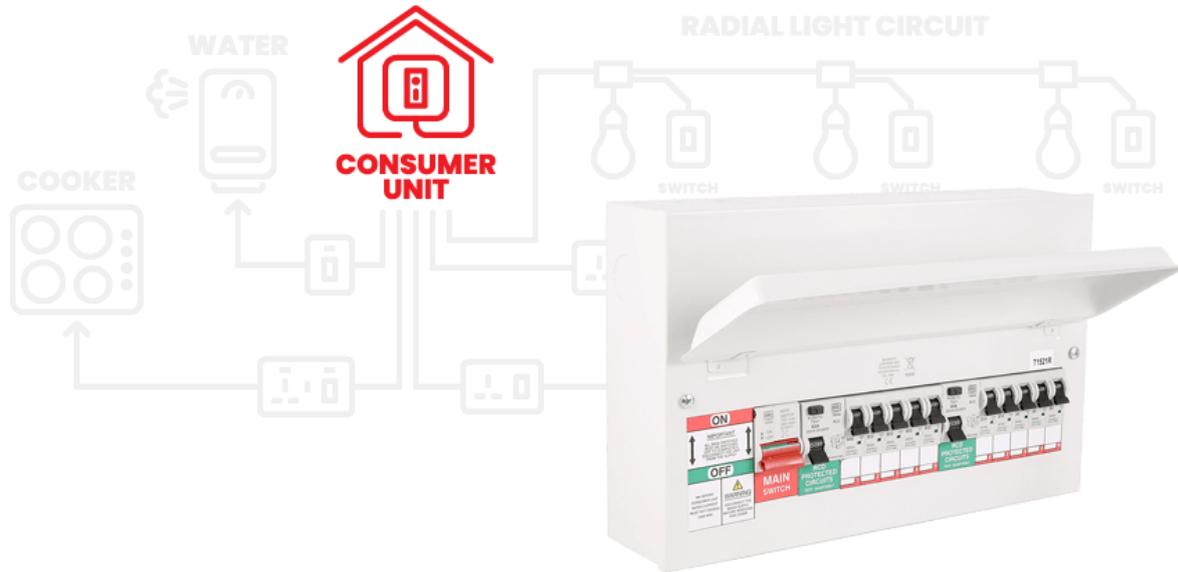
The consumer unit or commonly known as fuse box is the heart of a home wiring installation. It is usually mounted near the energy meter. A modern consumer unit as pictured above houses modular electrical devices called circuit breakers. There are 4 main kinds of circuit breakers in a common household: Main switch, MCB and RCD.
