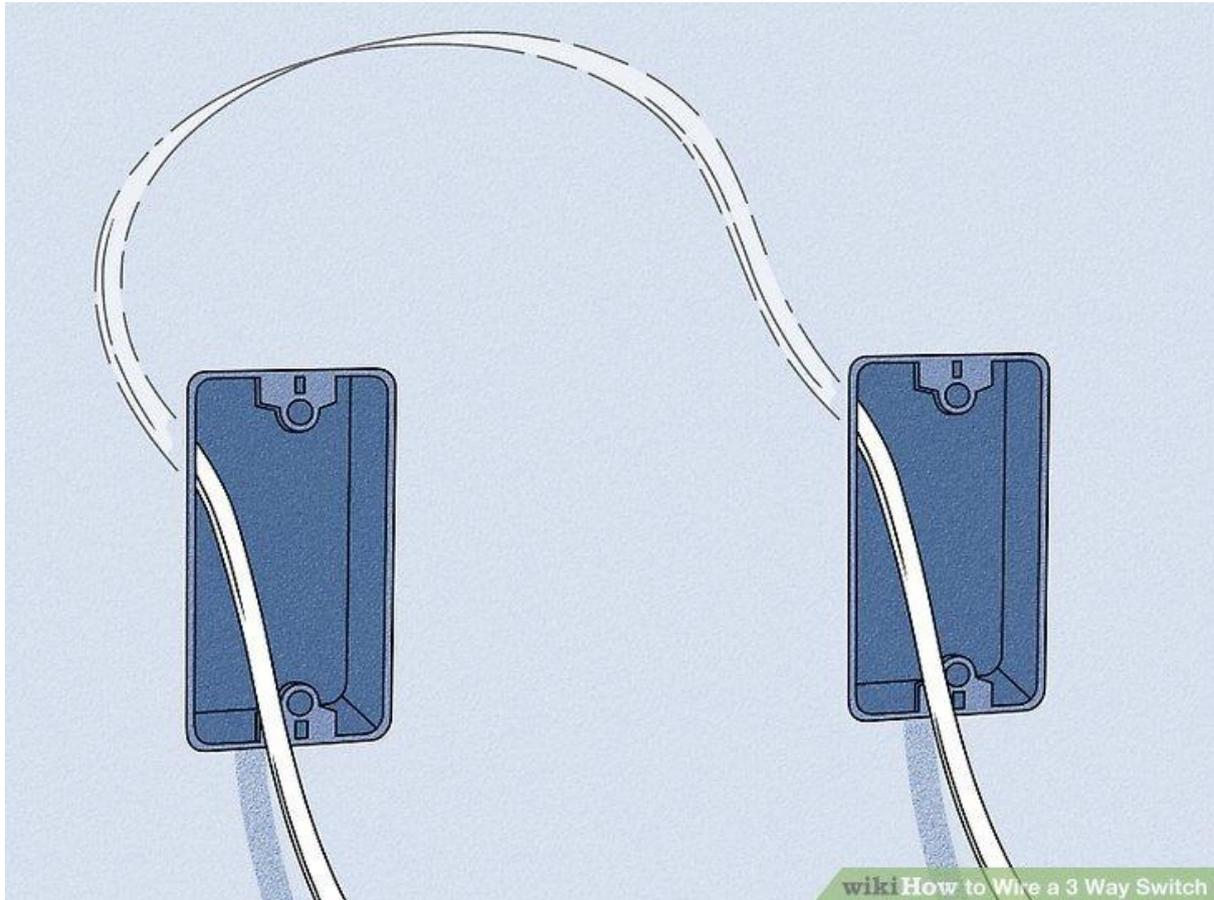
**Run 2 2-wire conductors between the two boxes.** Choose 14-2 or 12-2 NM cable, depending on the breaker.<sup>[5]</sup> 14 gauge wire needs a 15 amp breaker, while a 12 gauge wire requires a 20 amp breaker. You'll be using the top conductor to run your hot wires and your neutrals while the bottom conductor will be used for your traveler wires.
