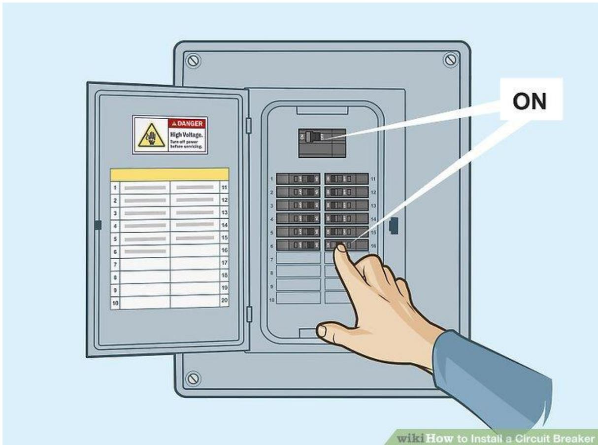
**Turn on the main breaker and test your new circuit breaker.** Standing to the side of the panel, restore power to the panel by setting the Service Disconnect or Main to "On" and then set the new circuit breaker to "On". Check for correct operation of the new circuit (light, outlet, etc.) with a test light or meter.<sup>[11]</sup>
