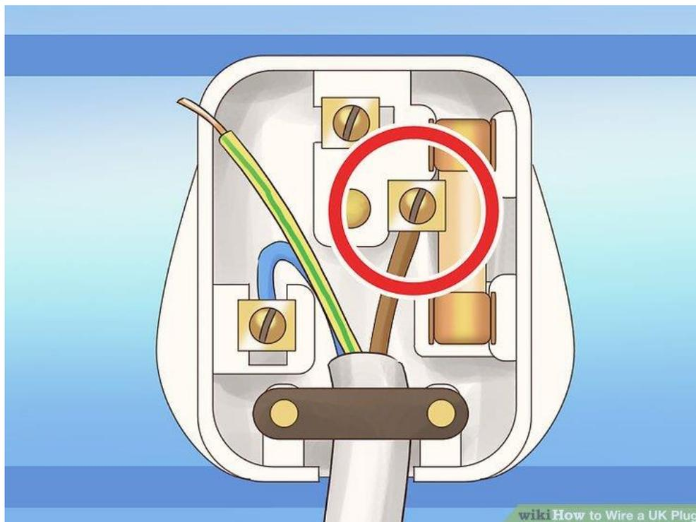
The Brown (Live) wire (br = bottom right) goes into the hole on the right, connected to the fuse (which should be clipped in).<sup>[4]</sup>
