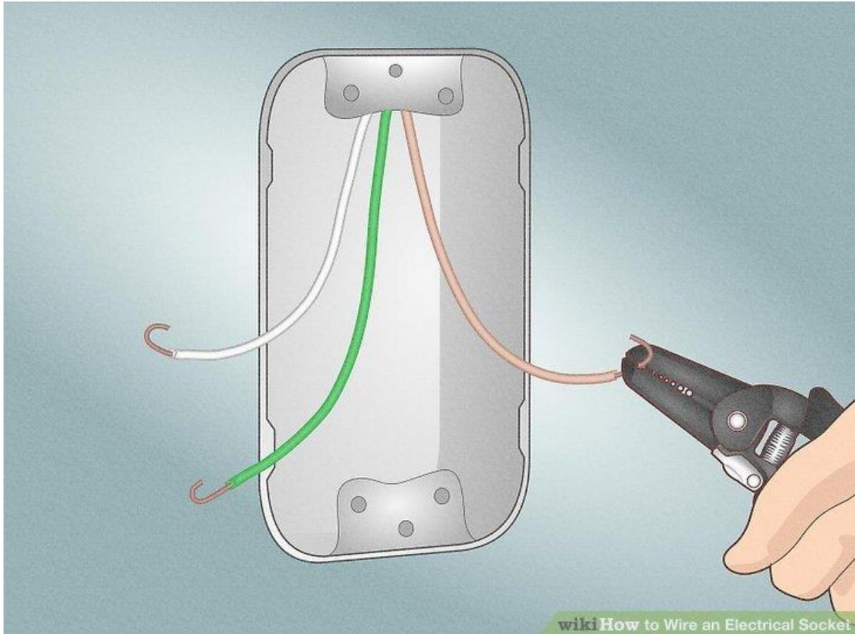
**Bend the wire ends into the shape of an umbrella handle.** The best way to secure your wires is to wrap them around the screw terminals. To prep for this, bend the stripped end into a U shape, so it will fit snugly around the whole screw.[\[16\]](#)
