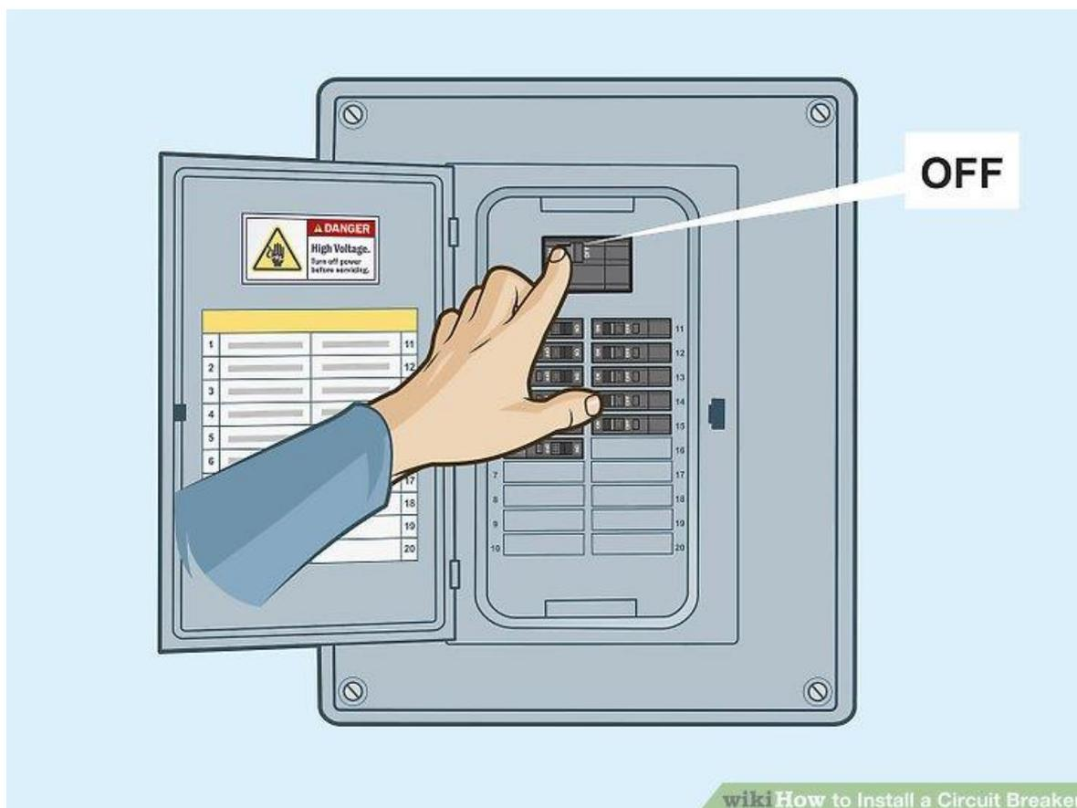
**Turn off the power supply to the electrical panel.** Locate the *Service Disconnect* or *Main* circuit breaker in the panel and set it to the "Off" position. This circuit breaker is likely to have the largest amp value and will be located either at the top or bottom of the panel.
