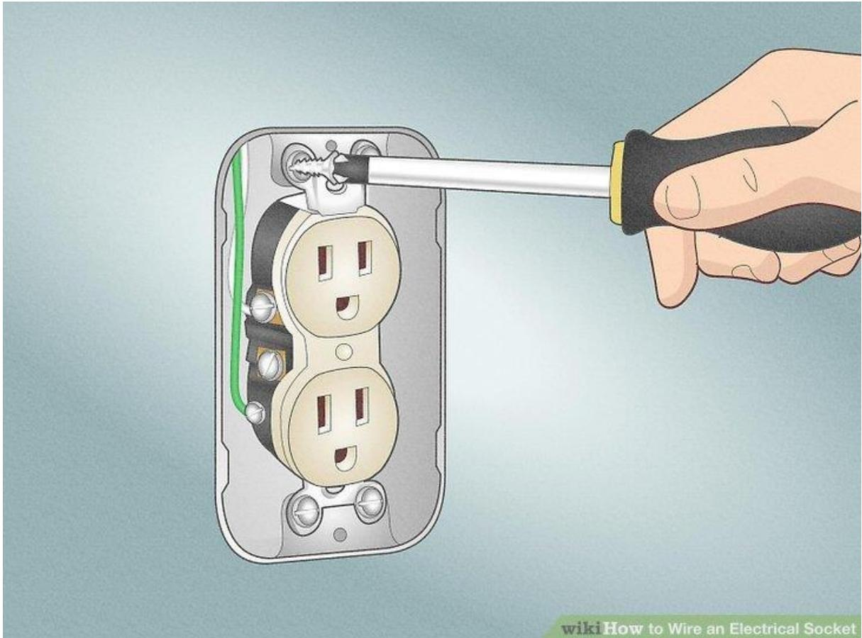
**Remove the old socket.** Once you are certain the power is off, unscrew the faceplate of the old socket and pull it out from the wall box. To detach the wires from the socket, unscrew the terminals just enough that you can slip the wire loop off of them.<sup>[8]</sup>
